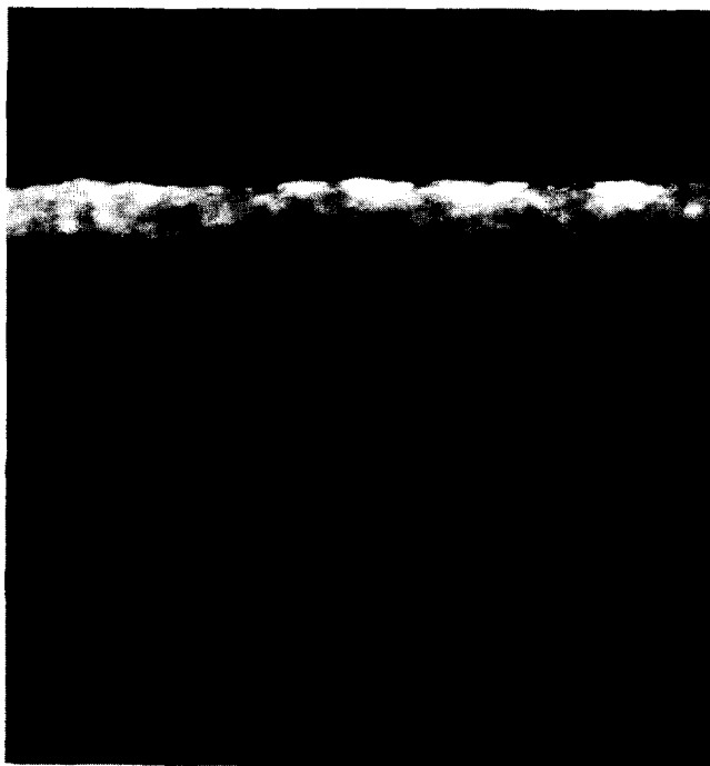
FIG. 1. Cross-sectional weak beam HVEM photomicrograph of the buried oxide layer in an as-implanted sample illustrating the heterogeneous nature of the unannealed top silicon layer.
