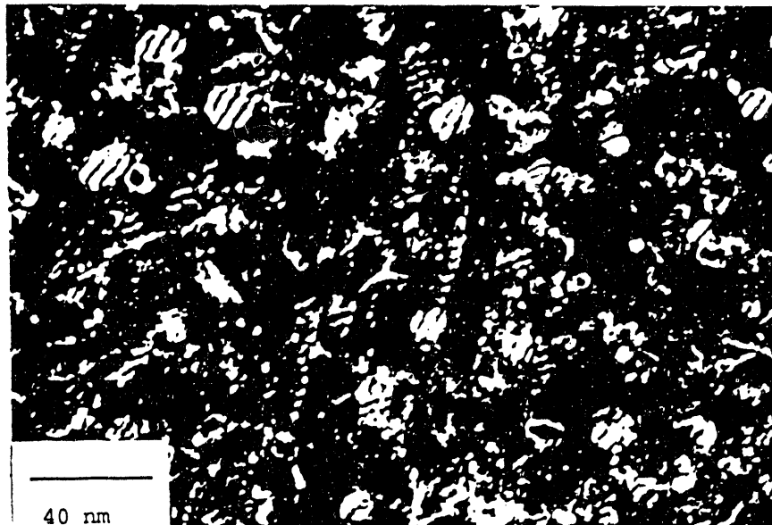
FIG. 3--Weak beam dark field micrograph of 304L SS ion-irradiated to 5 dpa
