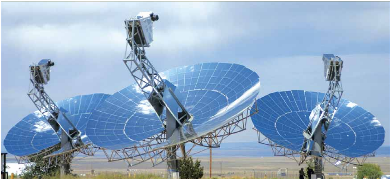
Solar dishes with sterling engines are a technology of major potential for low-density locations, suitable for public spaces within suburbia. Credit: Tessera Solar.
