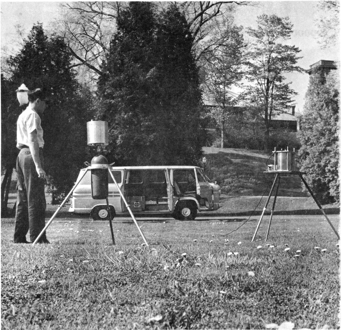
Figure 2. The HASL pressurized ionization chamber and spectrometer set up for a typical measurement. Saratoga Springs, N. Y., 1963.
