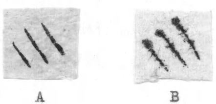
Fig. 4--Brush stroke test on cotton paper: (A) sized and (B) unsized.
