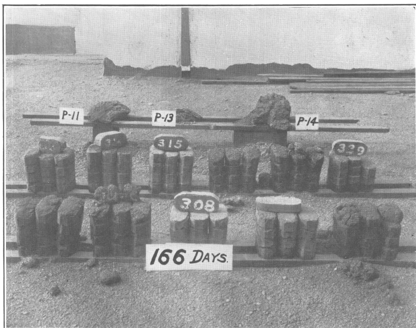
B. BRIQUETS AFTER EXPOSURE FOR 166 DAYS.
