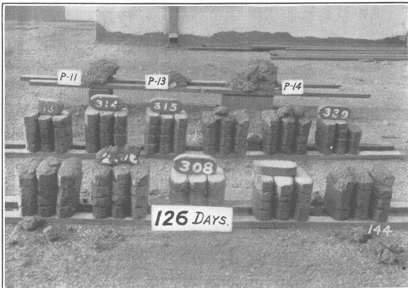
A. BRIQUETS AFTER EXPOSURE FOR 126 DAYS.
