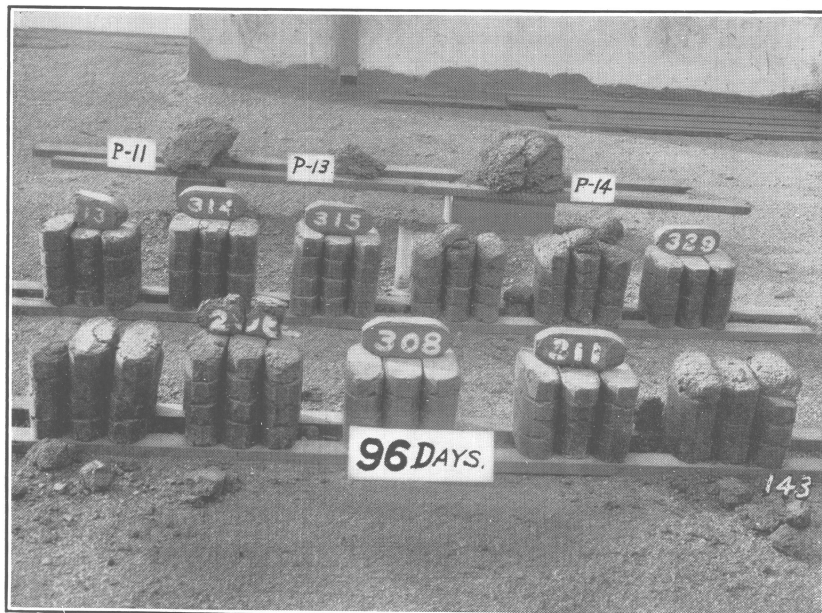
B. BRIQUETS AFTER EXPOSURE FOR 96 DAYS.
