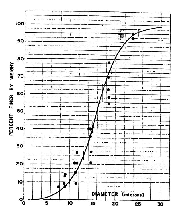
Figure 1. Malvern Calibration Test Results. ARC Data (Points) Versus NIST Standard Glass Beads (S-Curve).
