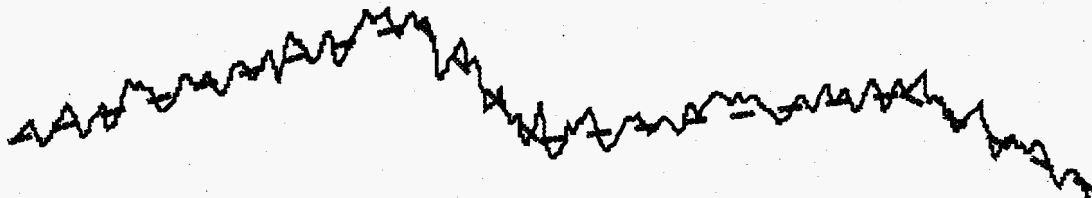
Figure 4: Sketch of a rough faceted surface. In addition to the high-frequency roughness, much larger facets, represented by the dashed lines, are also visible. The DWBA may fail for such surfaces.
