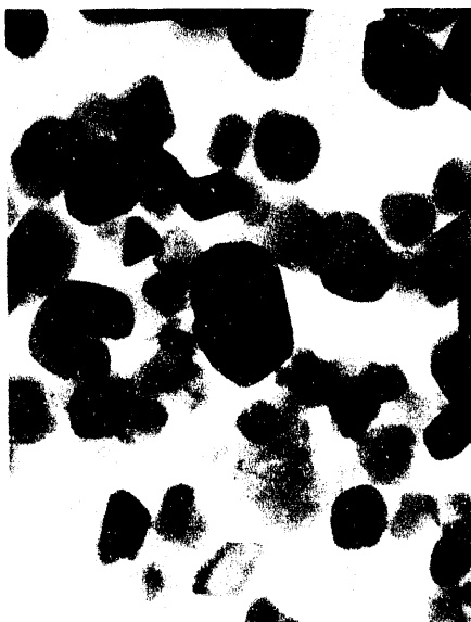
This typical high-surface, highly crystalline, nanoscale powder (highly magnified) was produced by using the RTDS process.
