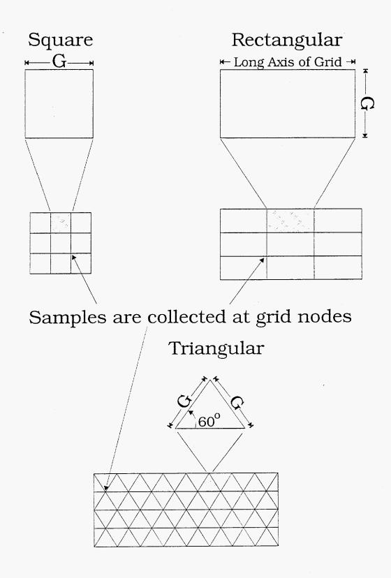
Fig. 2. Grid configuration for finding hot spots.
