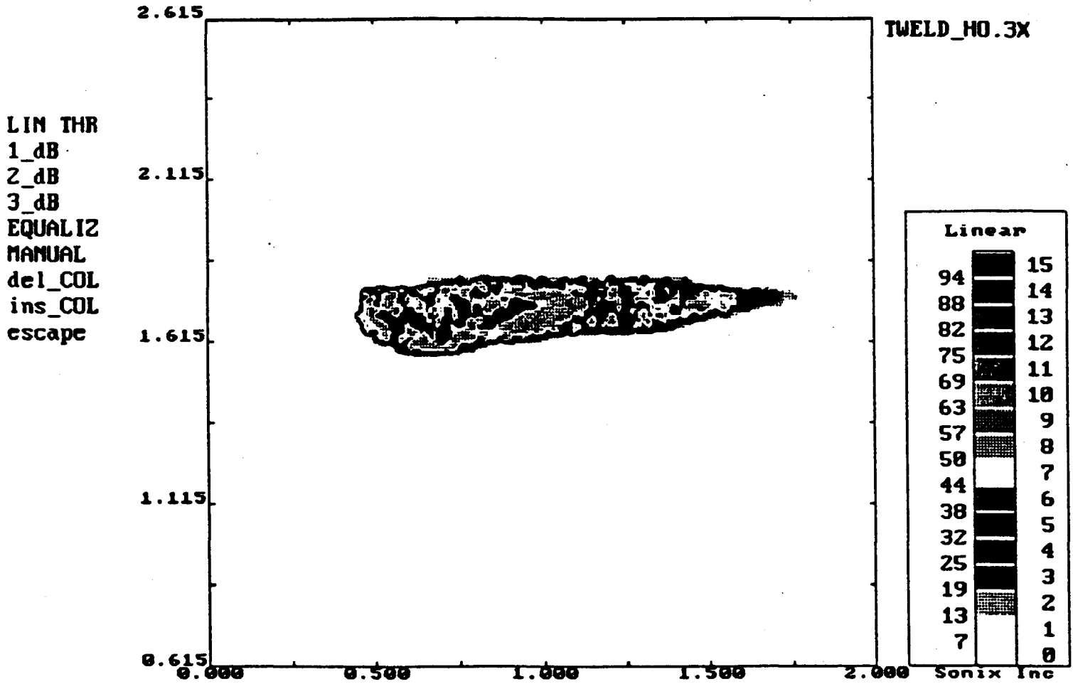
Figure 4. IR image of the surface temperature distribution on a SS sample with a defect during a 1.6 kw YAG laser welding. The defect was simulated by a subsurface hole of 2mm diameter along the laser path. The right side of the image shows the hot spot caused by the hole.
