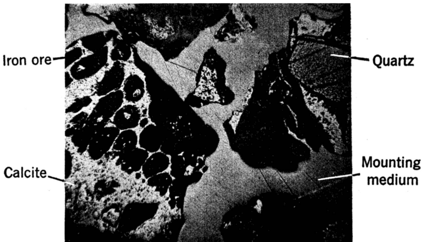
FIGURE 22.—Photomicrograph of Spaulding mill feed, showing locking of iron ore in the form of oölites (essentially hematite) with calcite. 5/16 inch = 48-mesh; X 40; reflected light. Minus 28- plus 48-mesh; sink, 2.9; float, 3.7.
