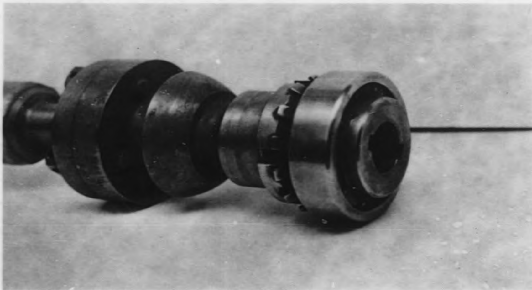
Single Rig Drive Shaft Showing Condition of Valve - Hours of Operation 1140
