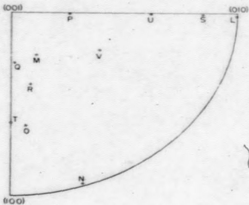
Figure 2. Quadrant of a (001) Standard Projection Showing the Crystallographic Locations of the Directions of Compression of the Eleven Crystals Studied.
