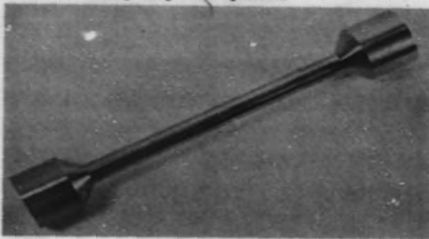
Figure 6. Zirconium Clad, Zirconium-4.3w/o Uranium Alloy Loop Test Specimen
