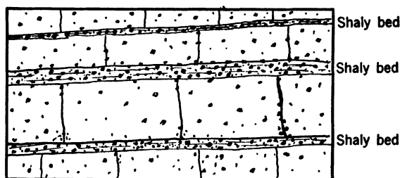
FIGURE 3.—Typical mineralization in 10-foot face of ore, southeastern Missouri.
