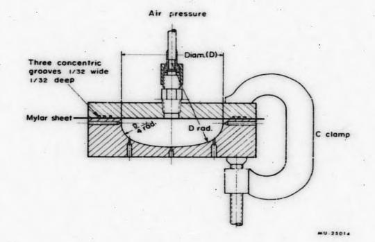
Fig. 2. Cross section of a mold for forming Mylar domes.
