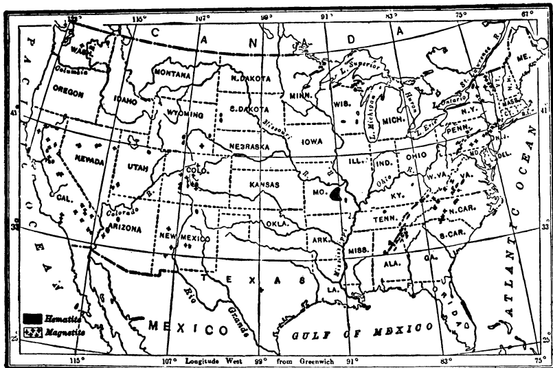
FIGURE 7.—Occurrence of hematite and magnetite in the United States, according to Harder (Ries).
