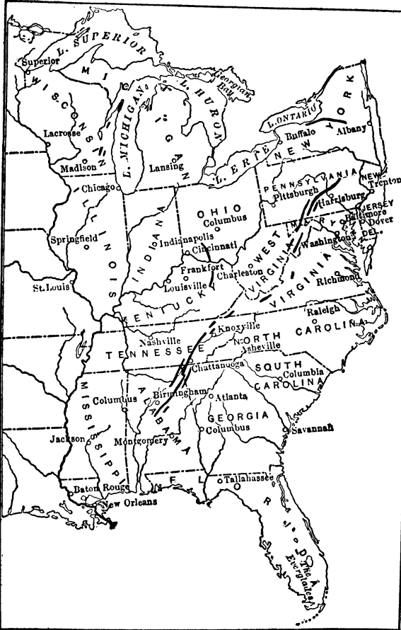
FIGURE 8.—Outcrops of Clinton or fossil iron ores in eastern United States, according to McCallie (Ries).
