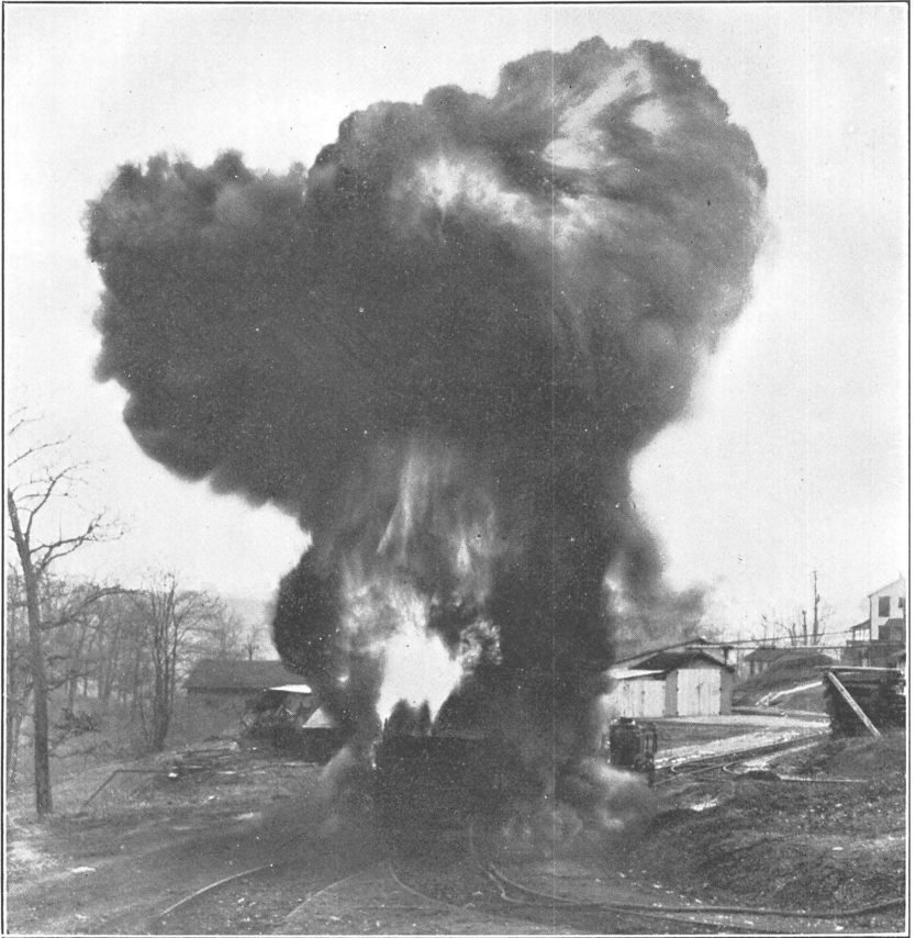
FIGURE 11. -Ignition of a coal-dust cloud in open air by an electric arc.
