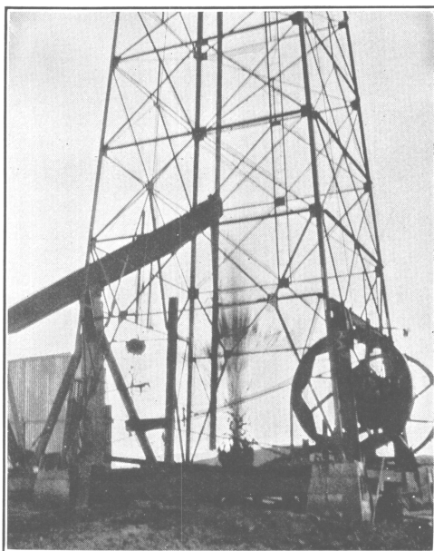
FIGURE 21.—Paraffin being blown from well after forming bridge with standard tools
