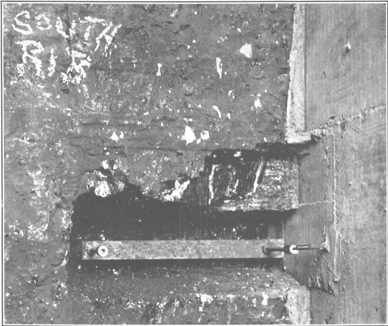
FIGURE 16.—Steel bar set in end of stopping 4 to measure end movement
