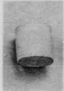
Fig. 16. Results of 500 Thermal Cycles (200 - 700° C) on Powder Compacted Uranium Alloys
