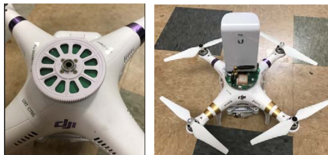
Fig. 4.29: Antenna assembly with DJI Phatom3 [26]
