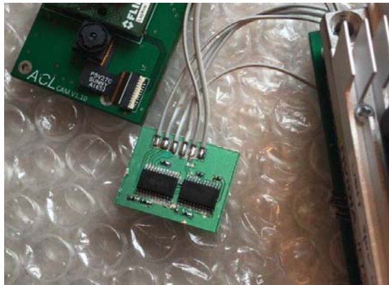
Fig. 6.14: Attached PCB for TCA9539
