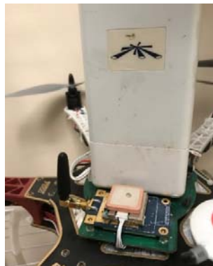
Fig. 3.10: Drone WiFi system twin-CPU platform
