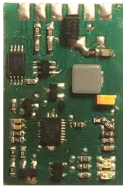
Fig. 4.21: BQ24103A PWM 3-stage Li-ion constant-current charger
