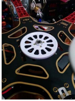
Fig. 2.4: Installation of gear on upper frame
