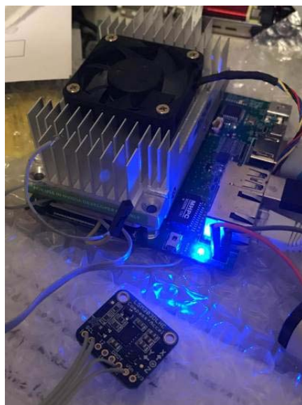
Fig. 6.15; TX2 V2.0 test with I2C LSM303
