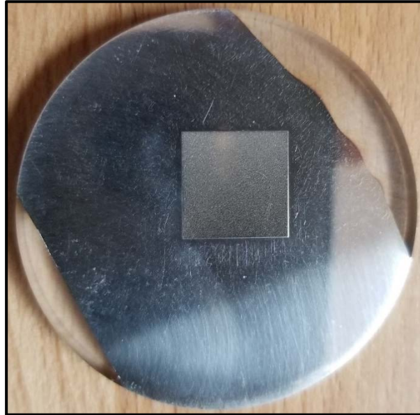
Figure 4.4: Acrylic Sample (Post Electron Beam Evaporation)
