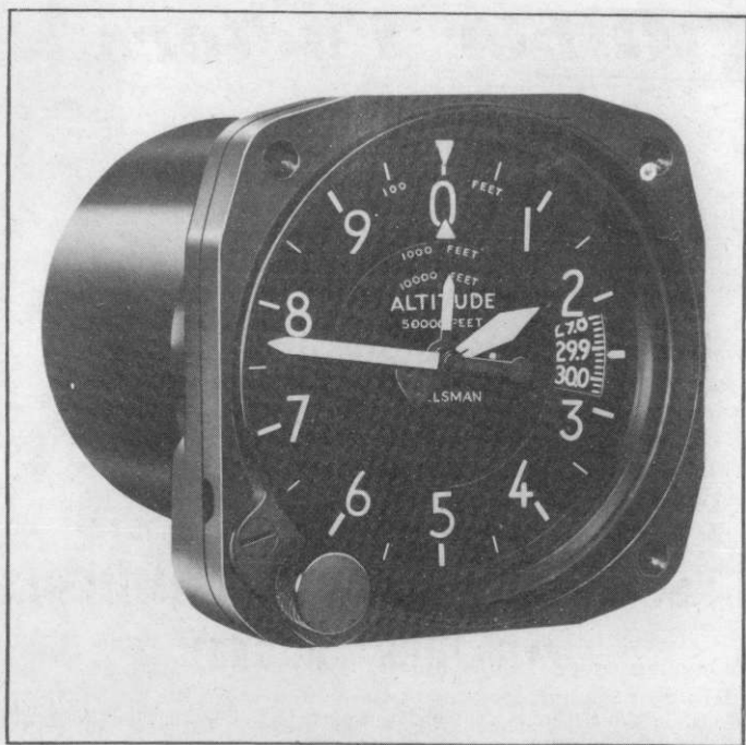
FIG. 1 - A TYPICAL ALTIMETER FOR AIRCRAFT.
