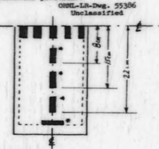
Fig. 1. Radial and axial positions at which power generation should be determined
