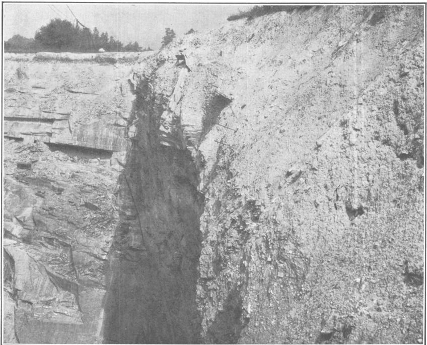
B. STRIPPING FACE LYING AT A STEEP ANGLE WITH ITS LOWER EDGE AT THE BRINK OF THE QUARRY.
