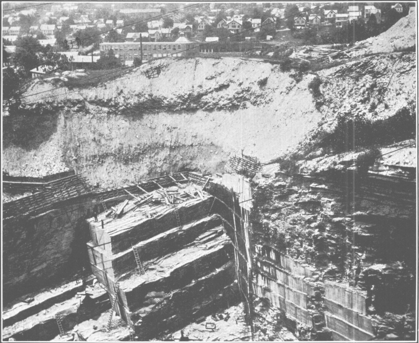
QUARRY SHOWING A MASS OF SLATE BLOCKED OUT FOR ONE YEAR'S OPERATION. (COURTESY OF NORTH BANGOR SLATE CO.)
