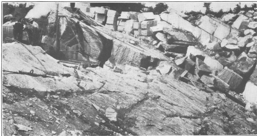
A. A QUARRY FLOOR SUITABLE FOR INCLINED-TRACK CHANNELING.
