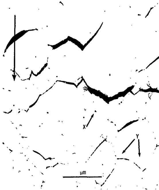
Fig. 11 Intergranular cracking in solution annealed Haynes alloy No. 25 pulled at 871°C. Section normal to gage 1/2-in. removed from fracture surface. Arrow indicates stress axis. The X marks the wedge-type void and Y the oval-type. Etchant: 100 ml HCl + 12 drops H 2 O 2 .
