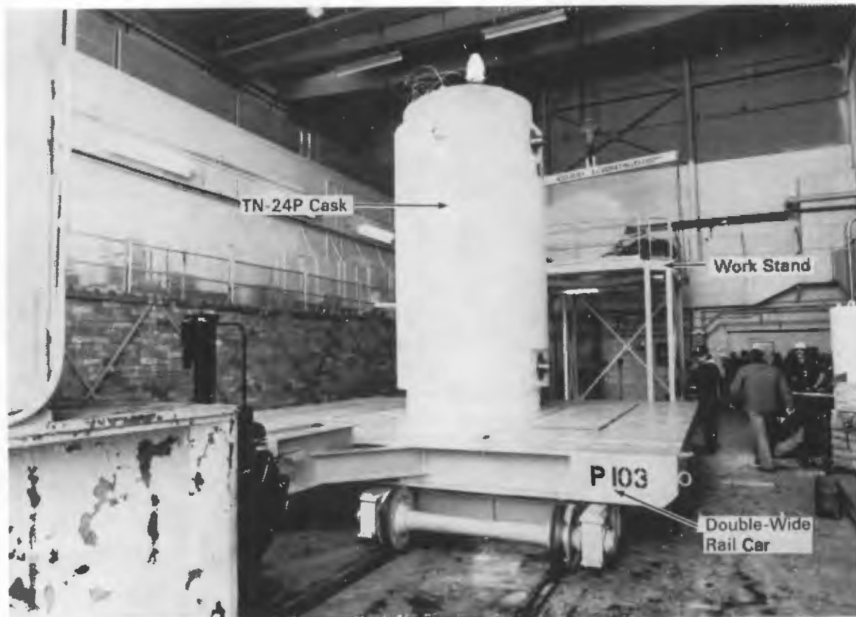
Figure 3-35. TN-24P Cask Being Moved to the Warm Shop Test Bay
