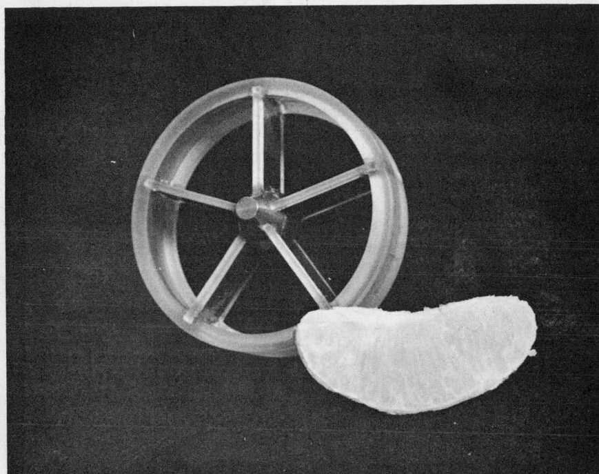
Fig. C14. The magnetic filter is made up of five magnets fixed into a radial geometry between a central lead plug and a lucite ring.
