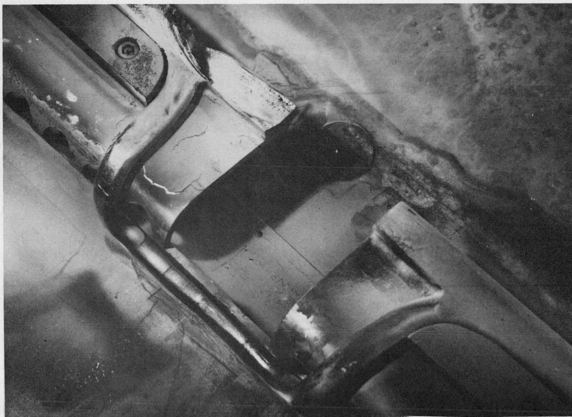
Fig. C11. Severe ion erosion of the dummy dee can be seen at the top of this photograph just left of center.
