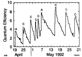
Figure 4. Quantum efficiency (750 nm and 120 kV) for first two activation cycles at the SLC injector. "A" indicates activation (heat cleaning/cesiation/fluoride), "C" indicates cesiation only. The initial QE had dropped to  $\sim 3.5\%$  by the time the plot began.
