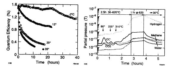
Figure 2. Temperatyre dependence of photocathode quantum effiviency lifetime.
