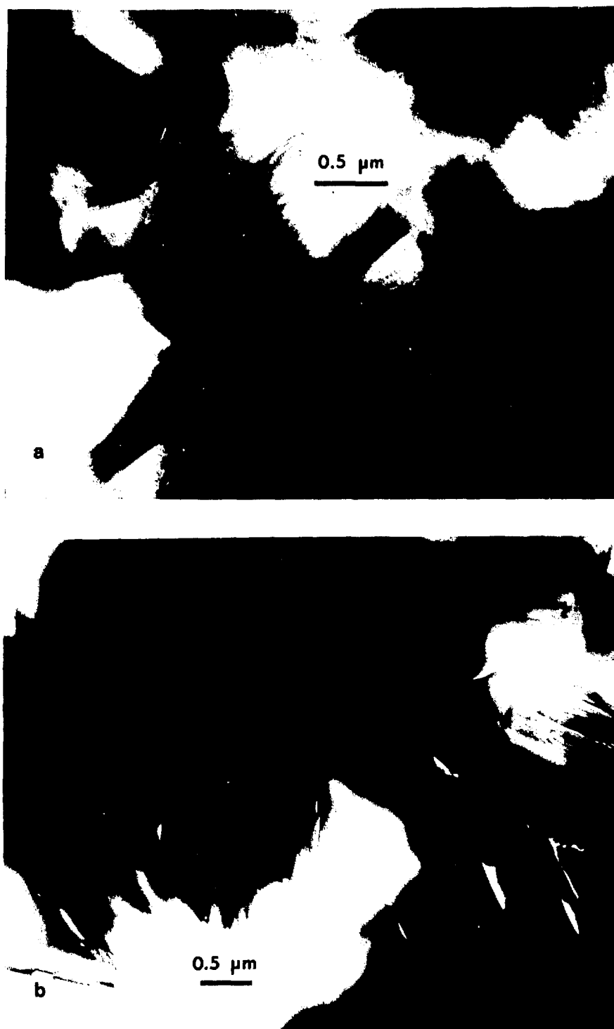
Figure 27. Transmission Electron Micrographs of Unirradiated (a) and Neutron-irradiated (b) DH Glass Ceramic. Note the irradiation-induced lens-shaped defects which formed between mica plates causing weakening of the material. 200 kV.
