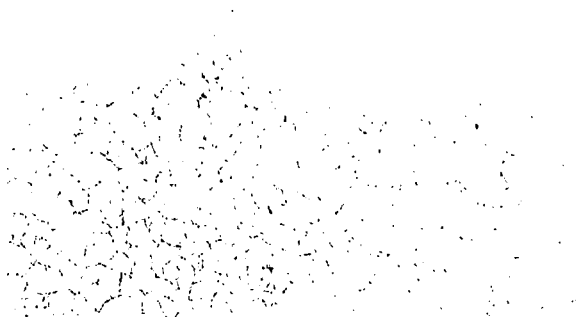
b. Defects patterns in blanchard ground surface
