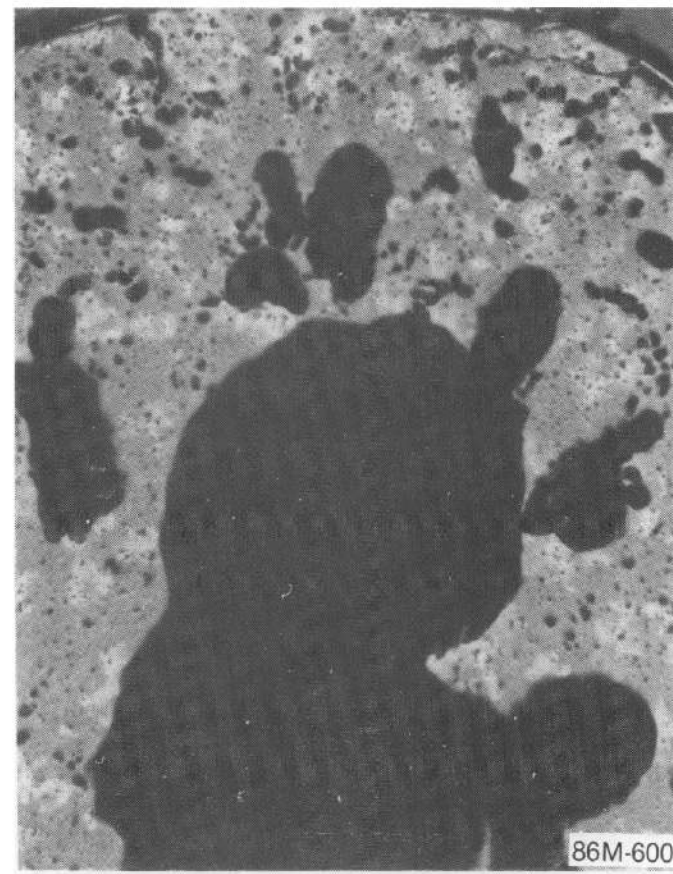
b. Photomicrograph of surface ceramic melt etched for zircaloy 100 μm
