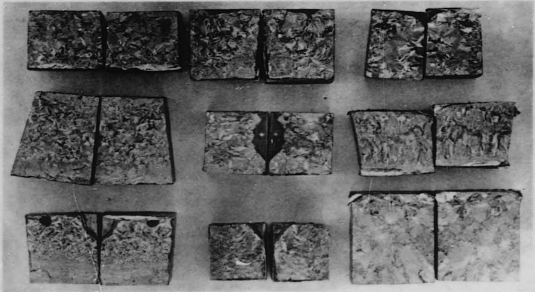
Figure 3k - Appearance of 3-Mil Spaced Brassments with Cu-20% Pd-3% In Filler Metal After 137 1/2 Hours of 600°F Corrosion Testing.
