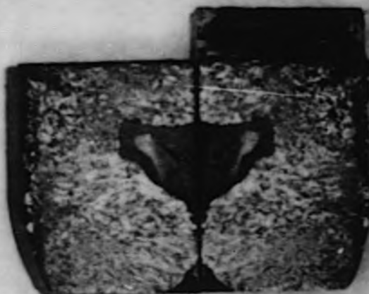
Figure 17 - Structure of 3-Mil Spaced Joint Brazed with Cu-4% Be Filler Metal.
