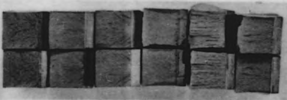
Figure 69 - Charpy Impact Bars Brazed with Zr-4% Be Filler Metal. Left three specimens broken at R.T.; Right two specimens broken at 550°F.
