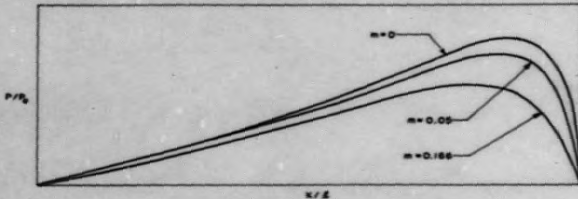
Figure 2. Pressure Distribution for Compressible Fluids along a Straight Slider Bearing
