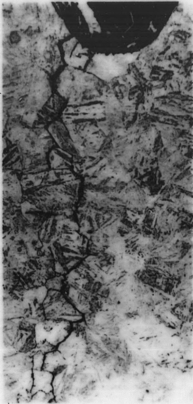
Figure 4. Intergranular Cracking in Thread of Laboratory Specimens 16E After 1000 Hr at 30000 psi and 1000 Hr at 58,000 psi. Rockwell Hardness C-40
