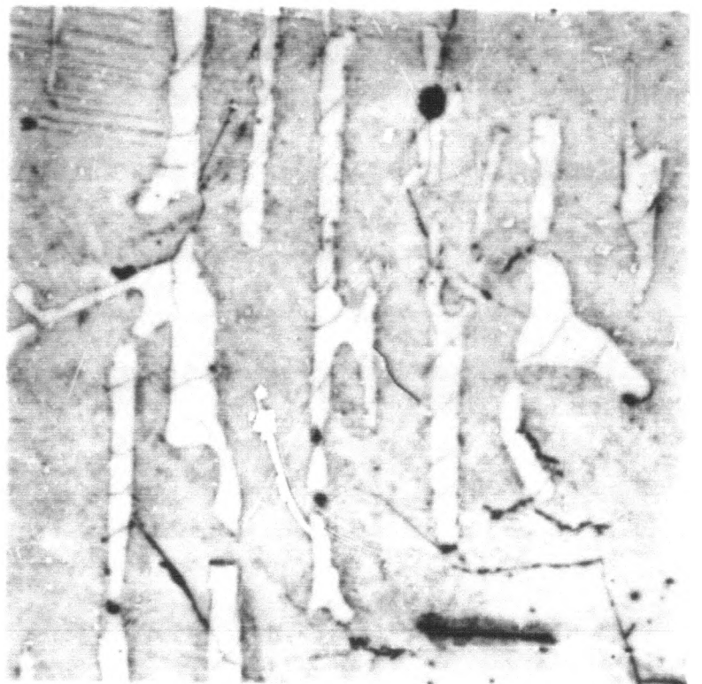
Fig. 9 - Y-74.9 wt pct Zn, furnace cooled, Nital etch, showing YZn_3 , light phase, in YZn_4 matrix, X100.
