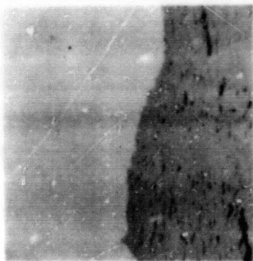
Figure 12. Intermetallic Niobium-Tin Embedded in Tin Matrix 100x, As Polished
