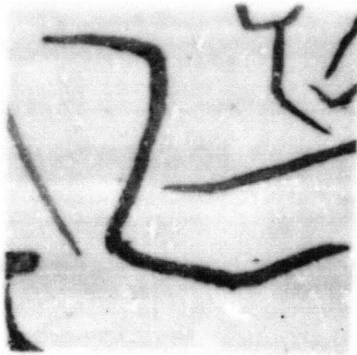
Figure 6. Grey Cast Iron 750x. As Polished
