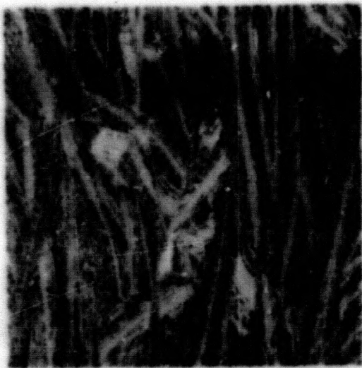
Figure 17. 42.5 w/o Cobalt-Zirconium 950x. Etch: HF-HNO 3 -glycerine
