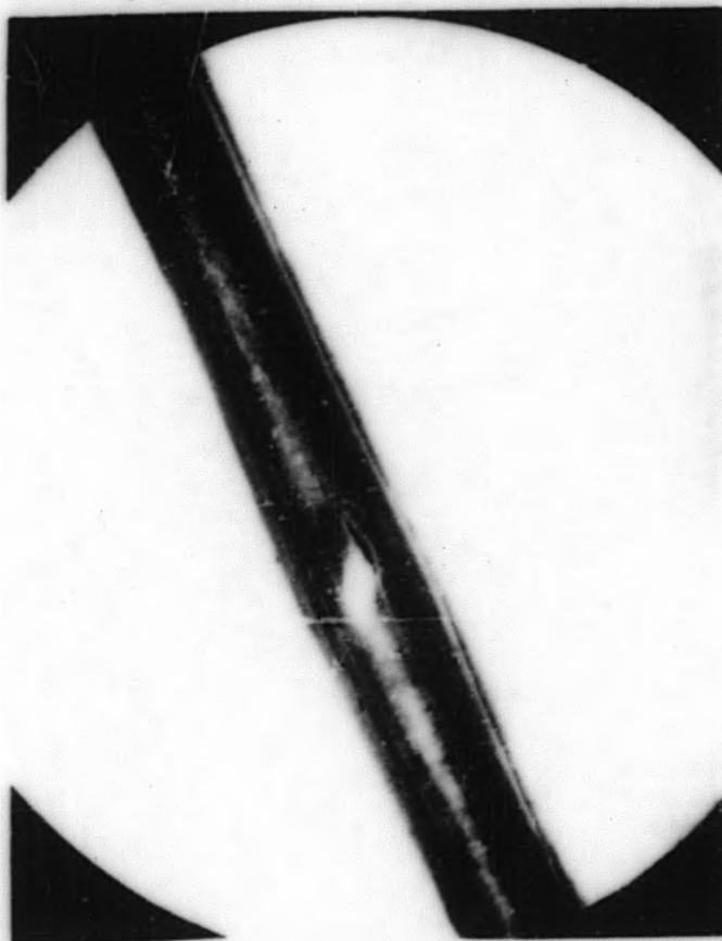
Figure 45. Burst Test Sample, Annealed HPD, Rod B Peak, 1 G
