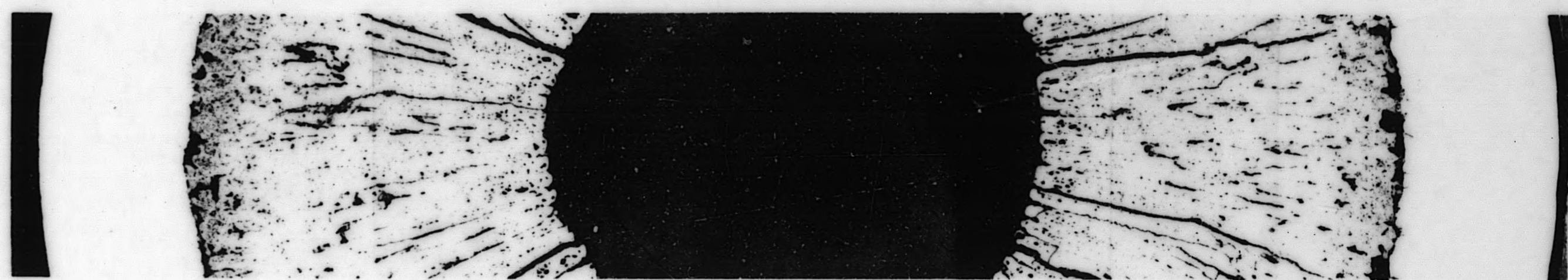
PRE-SODIUM MICROSTRUCTURE (AS POLISHED)
