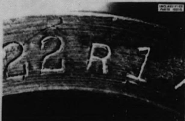
Fig. 40. Intake Hub of Impeller After Pumping Slurry Containing 78 g of Uranium per Liter for 100 hr at 250°C. There was no evidence of erosion. Original magnification 10X. Reduced 52%.
