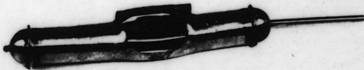
Fig. 26. Ruptured Titanium Plummet No. 1. Wall thickness, 0.025 inch.
