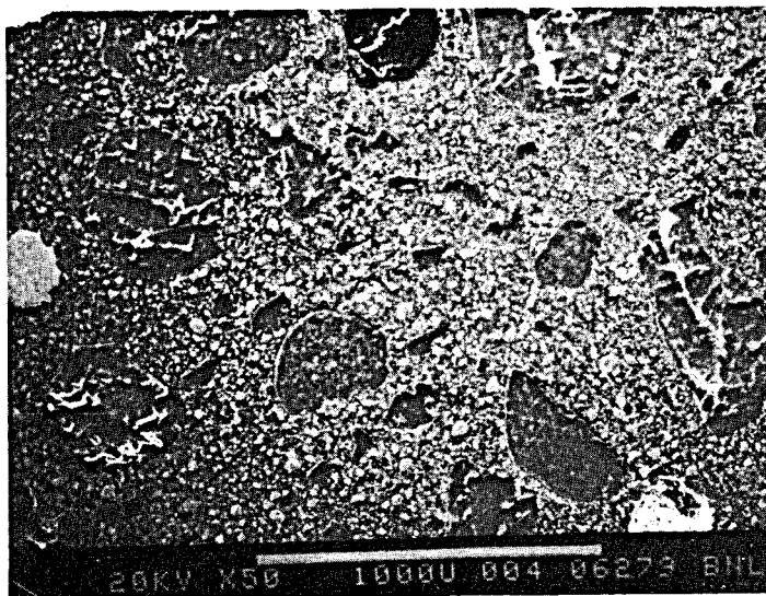
Figure 32. Effect of sand content in aggregate on the structure of PC.
