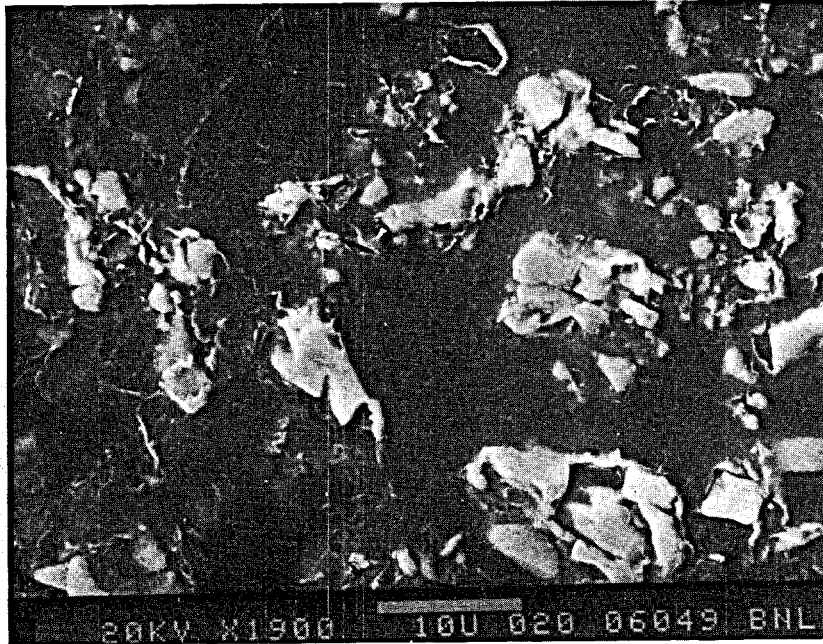
Figure 29. Scanning electron microscope picture of fractured surface of PC sample containing a 27.5% polymer loading.
