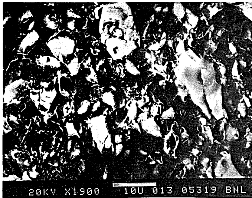
Figure 26. Scanning electron microscope picture of fractured surface of PC sample containing a 15% polymer loading.
