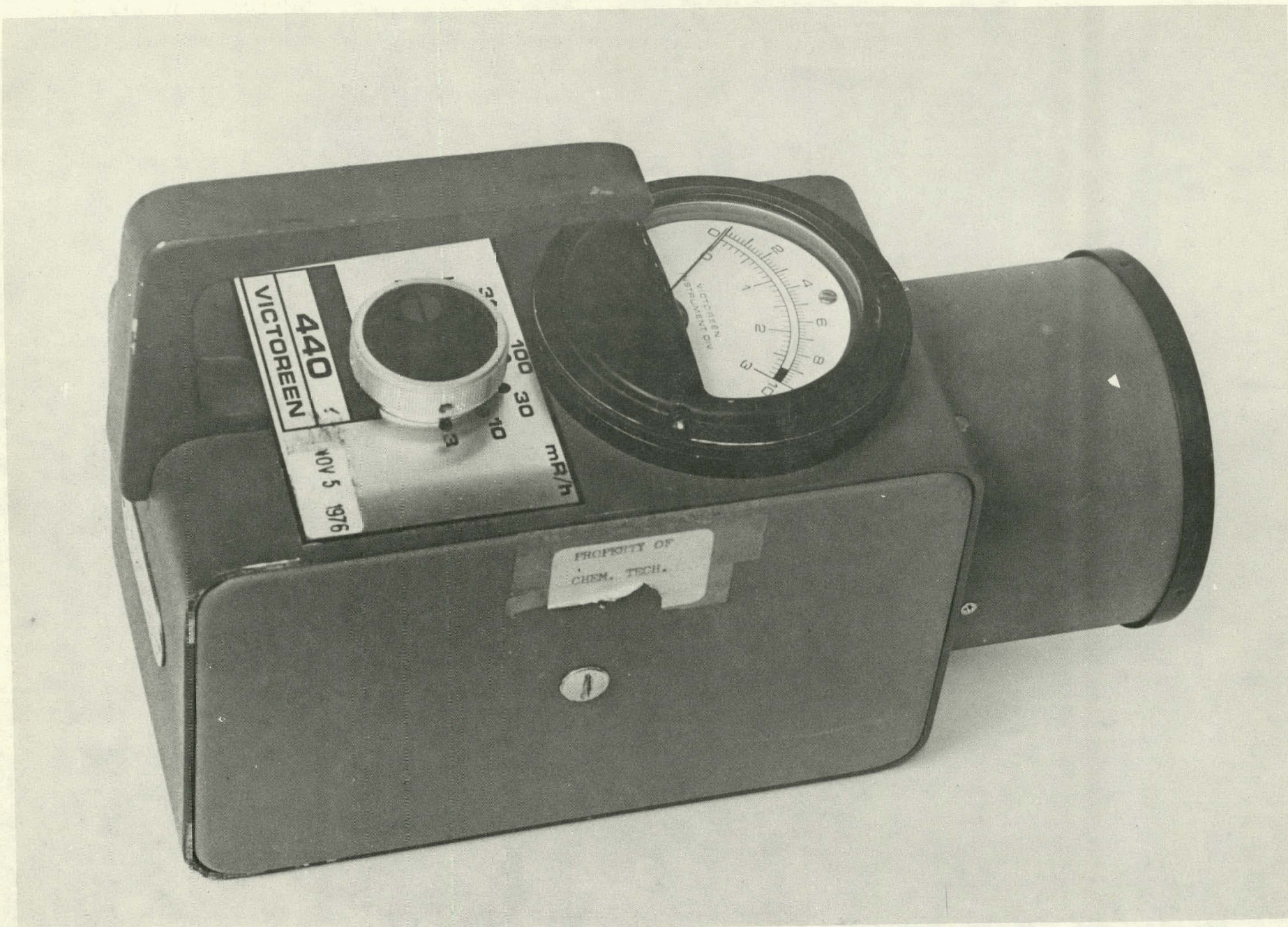
Fig. I-B. Victoreen Model 440 Ionization chamber.
