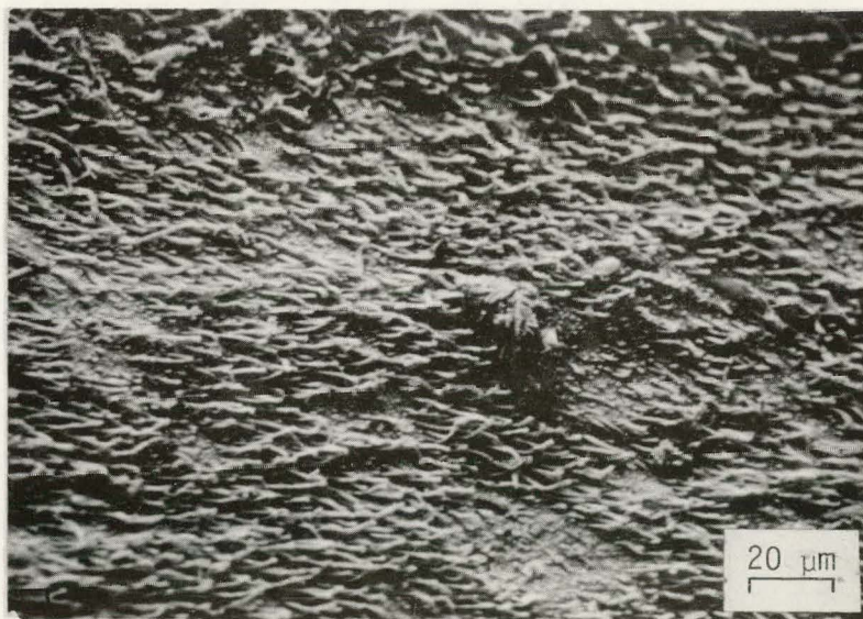
b. Shadowing of Blistered Surface by Protrusion
