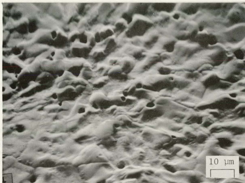
Exposed Side - Helium Blisters
