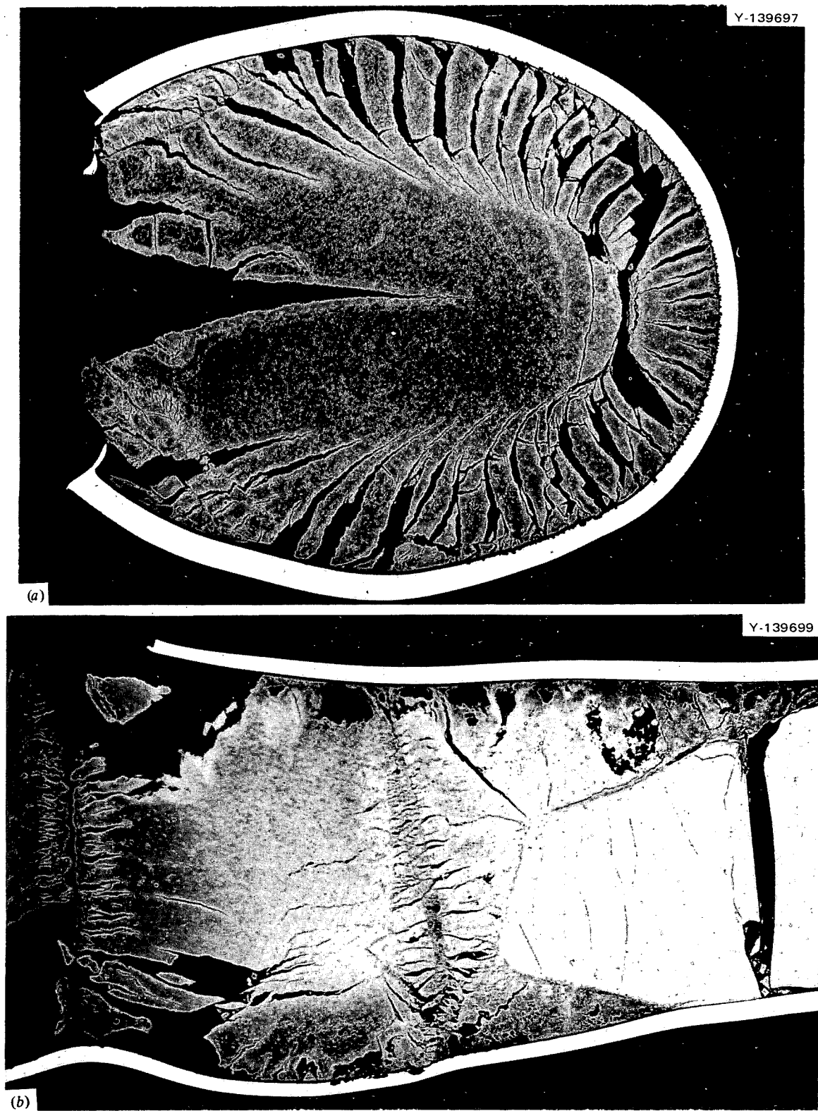
Fig. 42. Metallographic transverse (a) and longitudinal (b) sections from the swollen region of the Implant Test No. 9 fuel rod.
