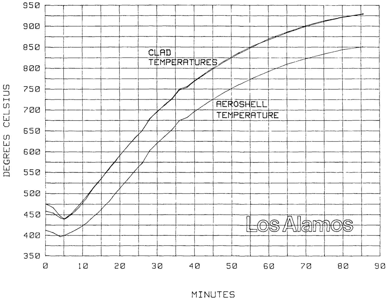
Fig. 19. Both instrumented clads in the DIT-3 test had the same self-heating thermal history before impact.
