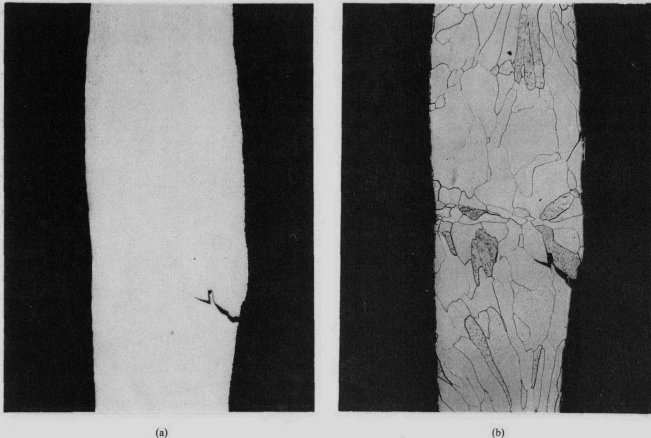
Fig. 12. The weld overlap region of capsule SRP-251 contained a large crack but only limited porosity. (a) As-polished. (b) Etched. (50X)
