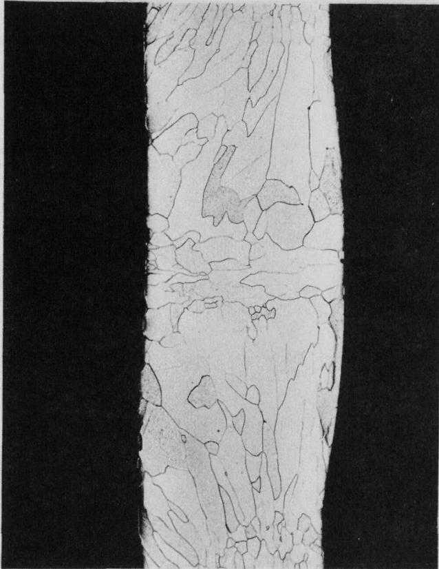
Fig. 8. The weld overlap region of capsule SRP-140 had a normal microstructure (50X).
