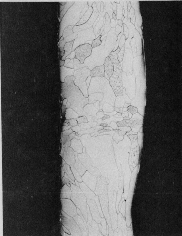
Fig. 17. The single-pass weld of capsule SRP-317 had a normal microstructure (50X).
