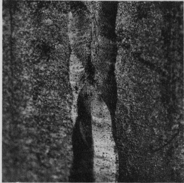
Fig. 6. Several fine cracks were visible in the weld overlap region just beyond the weld submergence in capsule SRP-140 (12X).
