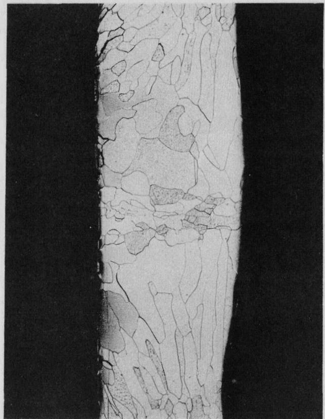
Fig. 9. The single-pass weld in capsule SRP-140 was normal (50X).
