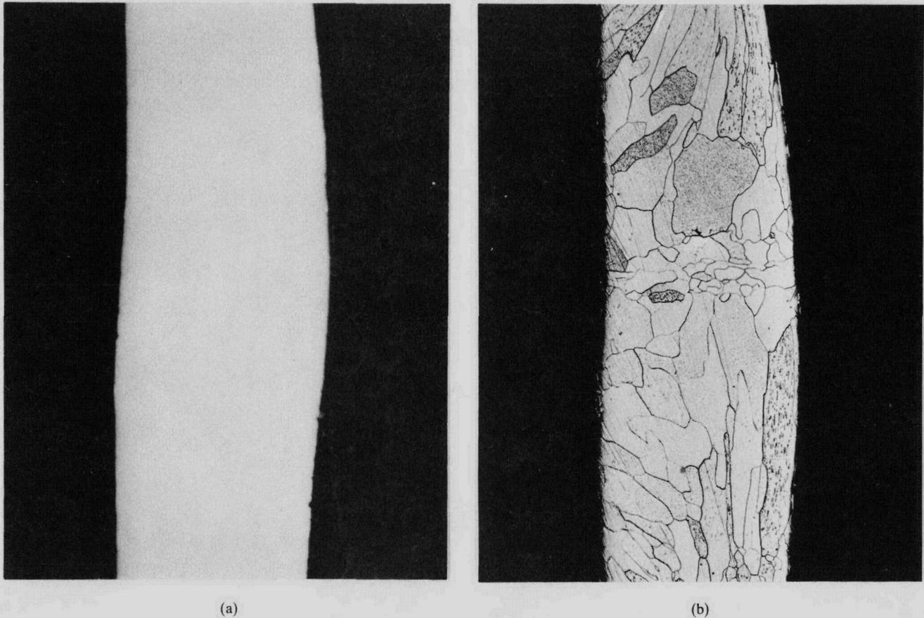
Fig. 13. The single-pass weld region in capsule SRP-251 was normal. (a) As-polished. (b) Etched. (50X)
