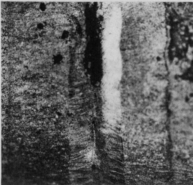
Fig. 11. The internal surface of the weld overlap region of capsule SRP-251 was rough and unreflective (12X).
