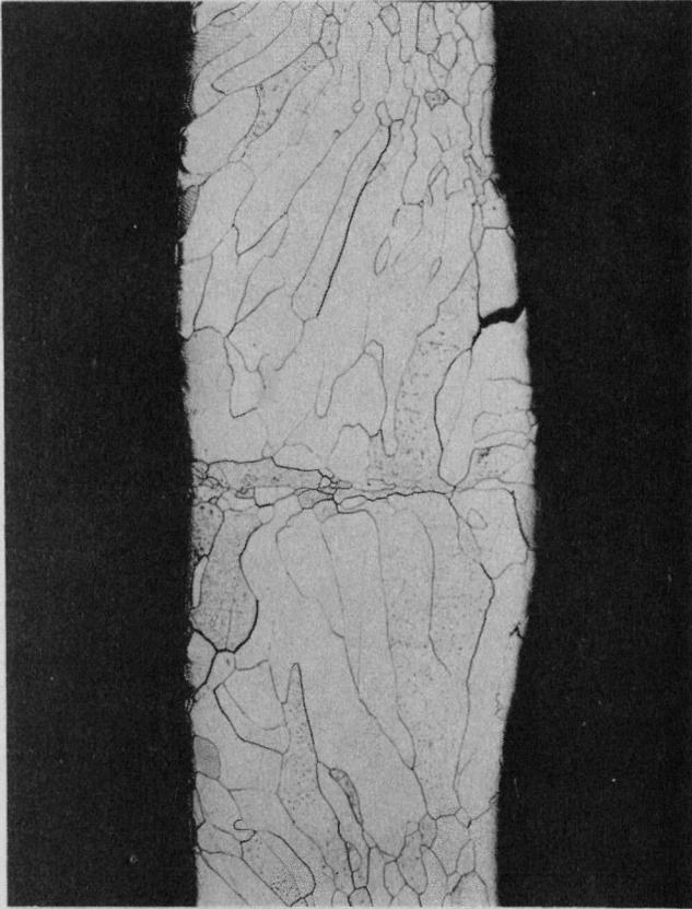
Fig. 16. The weld cracks are visible in this cross section of the weld overlap region of capsule SRP-317 (50X).
