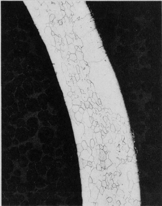
Fig. 5. Two very large grains were found on the outside of the radius of the vent cup from capsule SRP-127 (100X).
