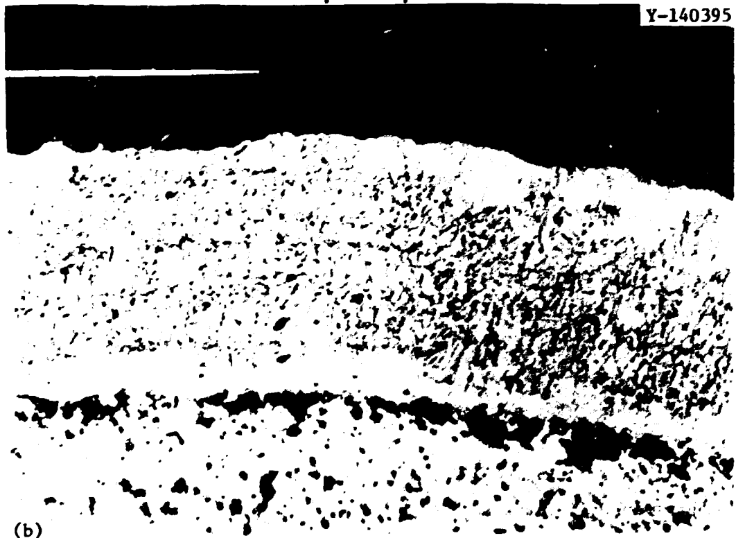
Fig. 4.9. Microstructures of Silicon Carbide Coatings from 0.13-m Coater. Deposition temperature = 1575°C, H 2 /MTS ratio = 45. (a) A-729, deposition rate = 0.26 \mu\text{m}/\text{min} . (b) A-743, 0.46 \mu\text{m}/\text{min} .
